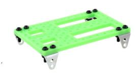
Insert both axles through the axle holders (top hole) and attach the gear and axle spacers. Do not attach the axle spacer on the gear side.
